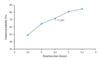
Figure 6. Emulsion stability of MES with variations of reaction times
