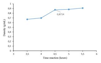
Figure 7. Density of MES with variations of reaction times
