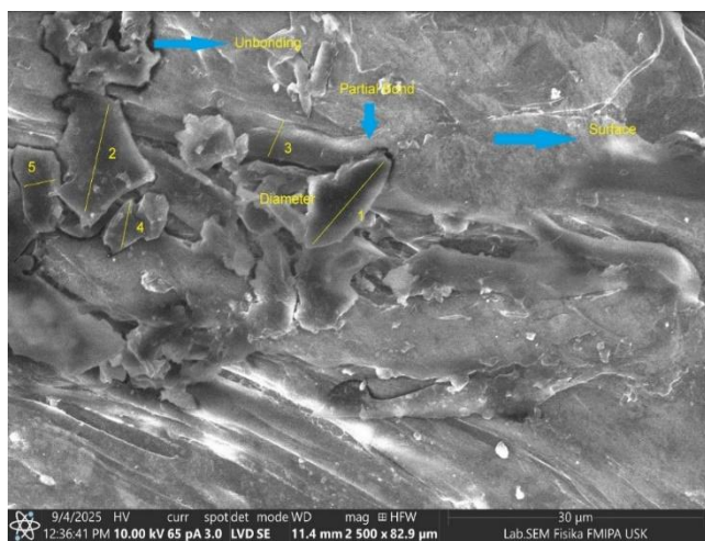
Figure 6. Surface Morphology of HDPE-Ramie Fiber
